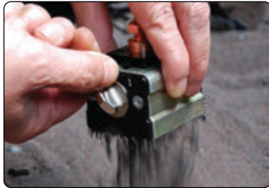
Turn OFF the PowerBase™ Grounding Magnet and metal chips fall away.
